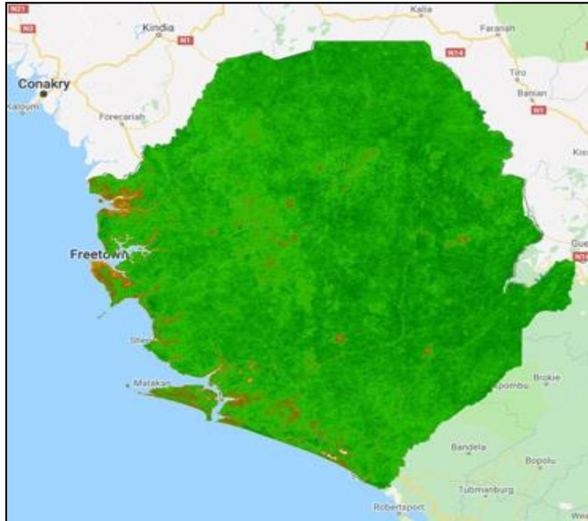
An example of NASA's MODIS 500 m 16-day Normalized Difference Vegetation Index product, nadir view. Combines both Terra and Aqua overpass for Sierra Leone.
