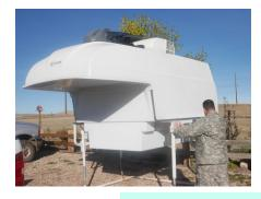
**Mobile Command Center -** Truck transportable, self-contained dual power, data storage, network control climate controlled work space. Auto-acquire SATCOM tracking and 50 MBps bandwidth. Input-Output ports for extended local communications
