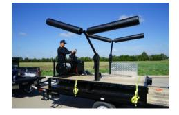
The Mooring Platform ~6' x 12', Turnkey operating base with power, helium, tools, winches; moved by forklift or helicopter; enables aerostat towing & two person operations; folds to fit ISO-20 container
