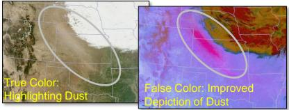
Multispectral remote sensing from VIIRS and MODIS for air quality and vegetation applications.
