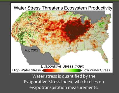
ECOSTRESS will provide critical insight into *plant-water dynamics* and how *ecosystems change with climate* via *high spatiotemporal* resolution thermal infrared radiometer measurements of evapotranspiration from the International Space Station (ISS).
