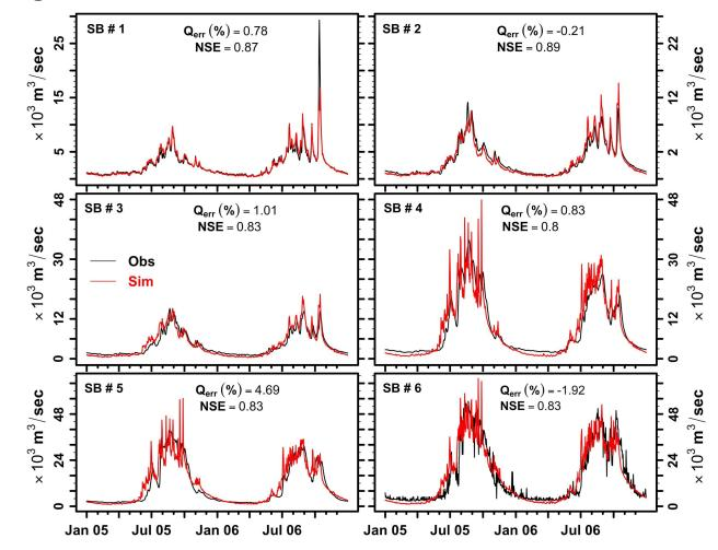
Daily simulated and observed discharge in m<sup>3</sup>/sec for the Lower Mekong River Basin (LMRB) at six sub-basin watersheds in calibration of the LMRB SWAT model excerpts from (Mohammed et al., 2018) 20
